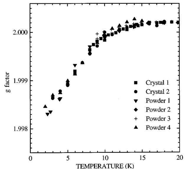
FIG. 4. Variation of the  $g$  factor below  $T_c$  of several powder and crystal  $K_3C_{60}$  samples measured at 225 GHz.
