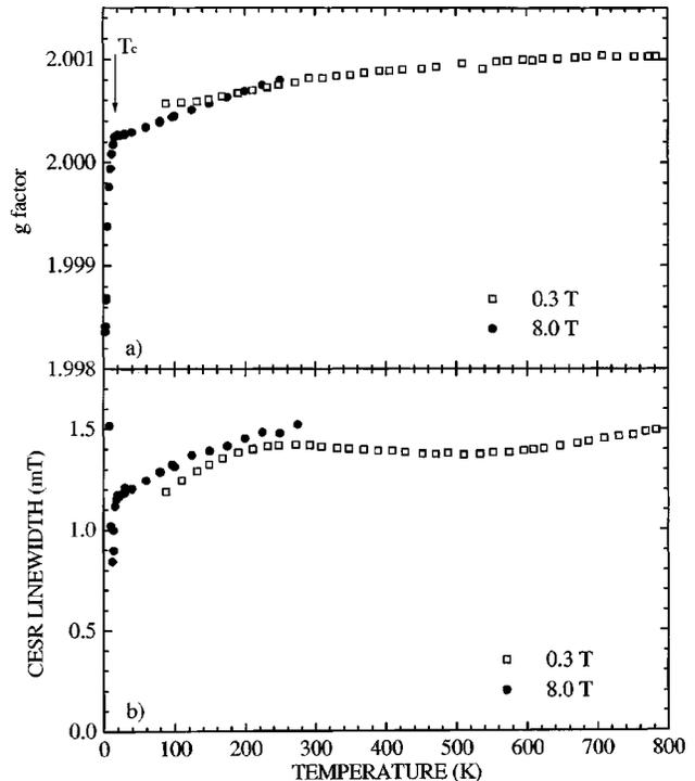
FIG. 1. Normal-state ESR properties of  $\text{K}_3\text{C}_{60}$ . (a) The  $g$  factor anomalously changes with temperature. (b) The linewidth measures the spin relaxation rate. Most of the changes are below 250 K (dots: 225 GHz; squares: 9 GHz).
