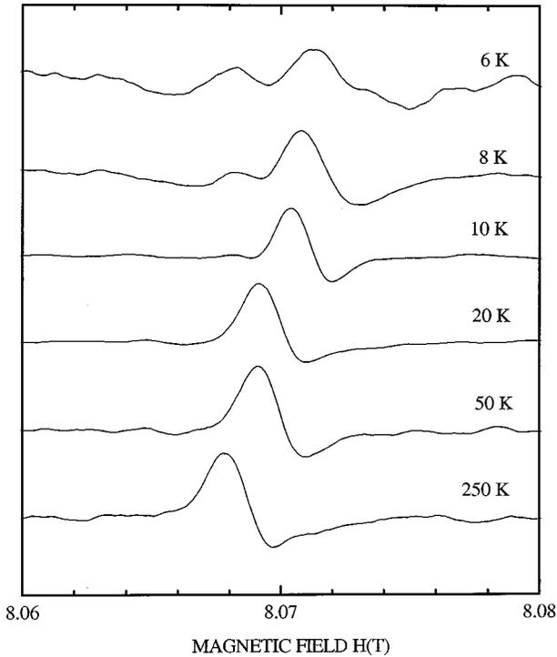
FIG. 2. Typical CCSR spectra of a  $K_3C_{60}$  crystal at 225 GHz. In the normal state the resonance narrows and slowly shifts to higher fields with decreasing temperature. Below  $T_c$  the resonance progressively shifts to higher fields and has a minimum linewidth at 10 K. At 6 K chaotic motion of vortices increases noise.
