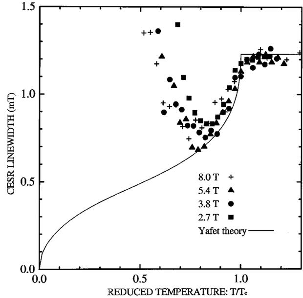
FIG. 3. CCSR linewidth vs reduced temperature of  $K_3C_{60}$  at various magnetic fields in the superconducting state. The sharp decrease of the relaxation rate below  $T_c$  is field independent. Below  $0.7 T_c$  the broadening is inhomogeneous. The solid line is the theoretical prediction of Yafet for scattering of normal excitations on nonmagnetic impurities.
