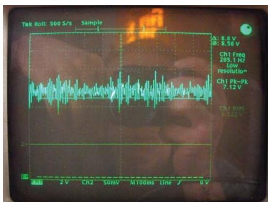
Figure 49: detector signal displayed on oscilloscope allow to measure the DC signal component of the detected light
