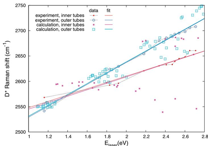
**Fig. 2** (online colour at: [www.pss-b.com](http://www.pss-b.com)) Raman D\* dispersion: comparison between theory and experiment.
